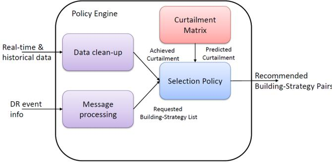
Fig. 4: Policy Engine components & data flow.
